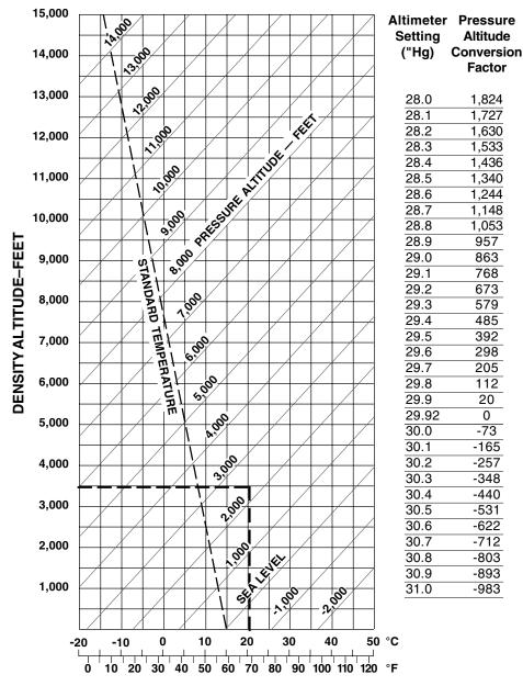
Example: Pressure altitude 2,200 (altimeter set at 29.92) Temperature 70° F = Density Altitude 3,500 ft.
